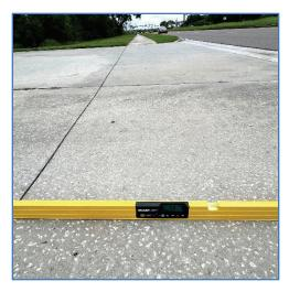
Photo 5 – First Baptist Church of Progress Village Driveway with a Cross Slope Greater than 5 Percent as Required to Meet ADA Standards
