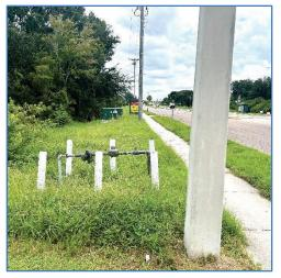
Photo 2 – Gas Line, Telecommunications, and Overhead Transmission Poles on the Back Side of Sidewalk
