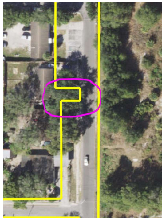
Figure 2 - Varying right-of-way of Segment A
