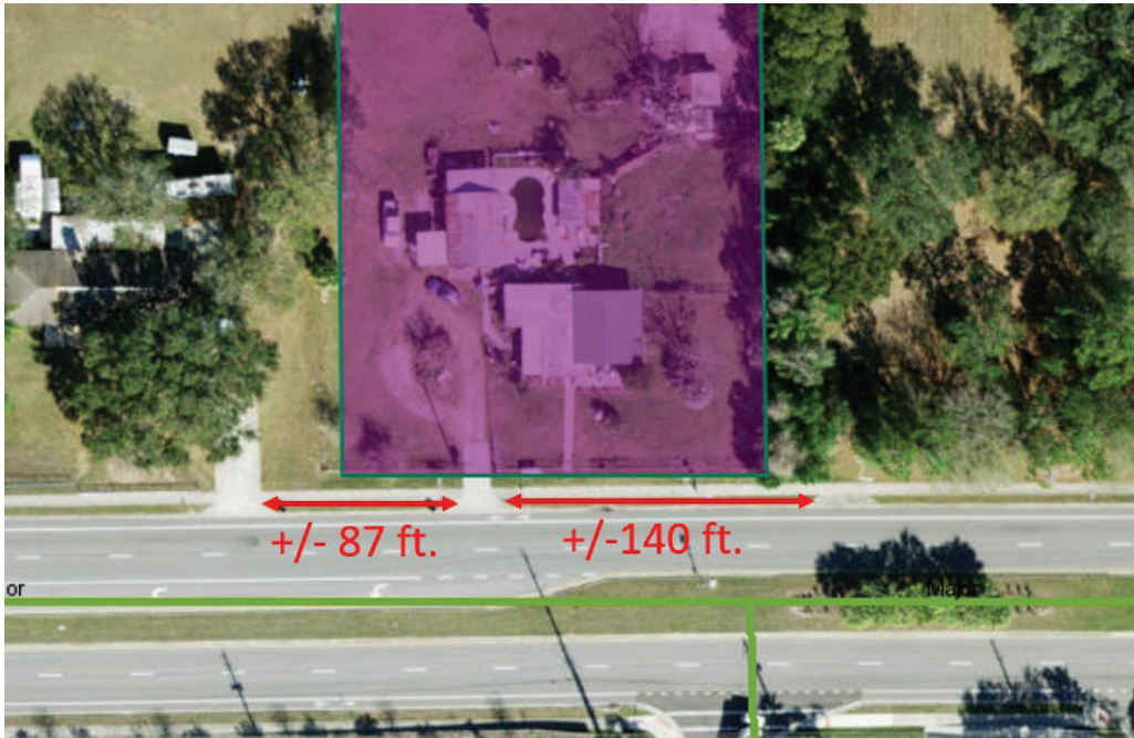
Photo showing spacing concerns on Boyette.
