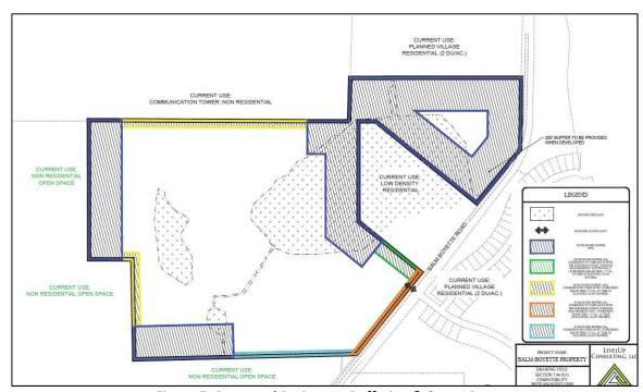
Figure 7: Proposed Perimeter Buffering & Screening
