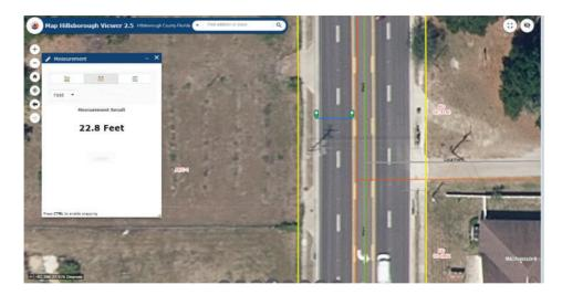
Figure 2. GIS Measurement of Hillsborough County's GIS Map showing an estimated lane width of distance of twenty-two feet.
