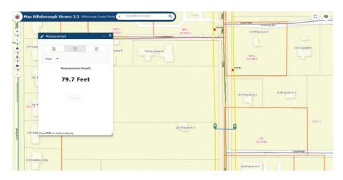
Figure 1. GIS Measurement of Hillsborough County's GIS Map showing an estimated ROW distance of eighty feet.
